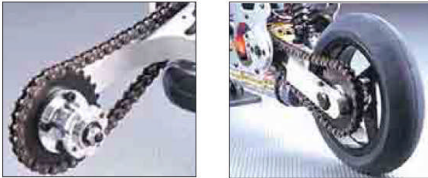
Rear wheel chain drive of a motorcycle
