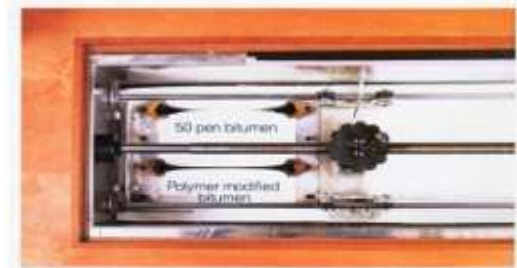
Photograph 3.2 – A plan view of the ductility test
