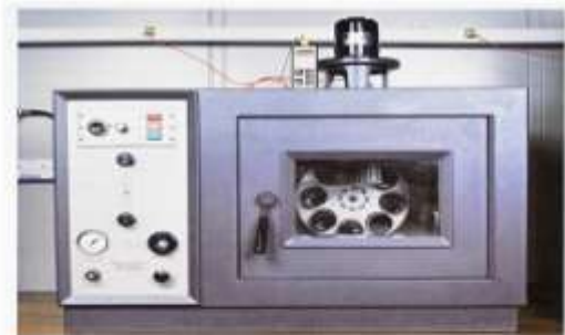
Photograph 3.3 – The rolling thin film oven test
