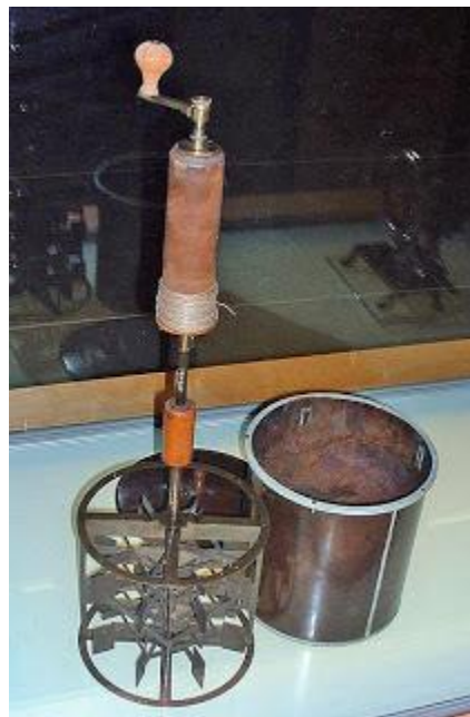
Joule's Heat Apparatus, 1845. [3]
