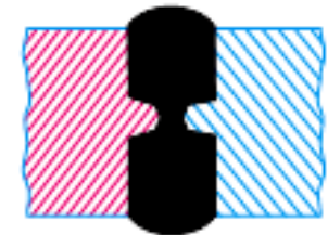
(e) Double U-butt joint.
