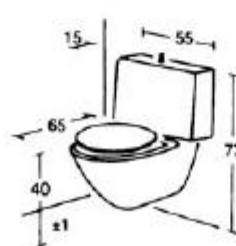
⑦ Wall-mounted deep-flush toilet bowl and cistern
