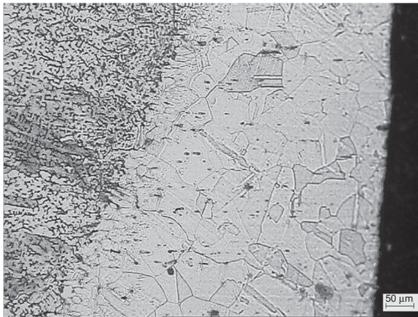
Fig. 6.1.9 Micrograph near the weld region of the sample showing equiaxed grains of austenite with annealing twins in the cone portion. Etchant: Aqua regia.
