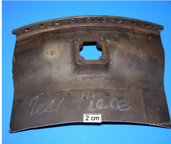
Fig. 6.1.1 Portion of the exhaust outer cone in the as-received condition.
