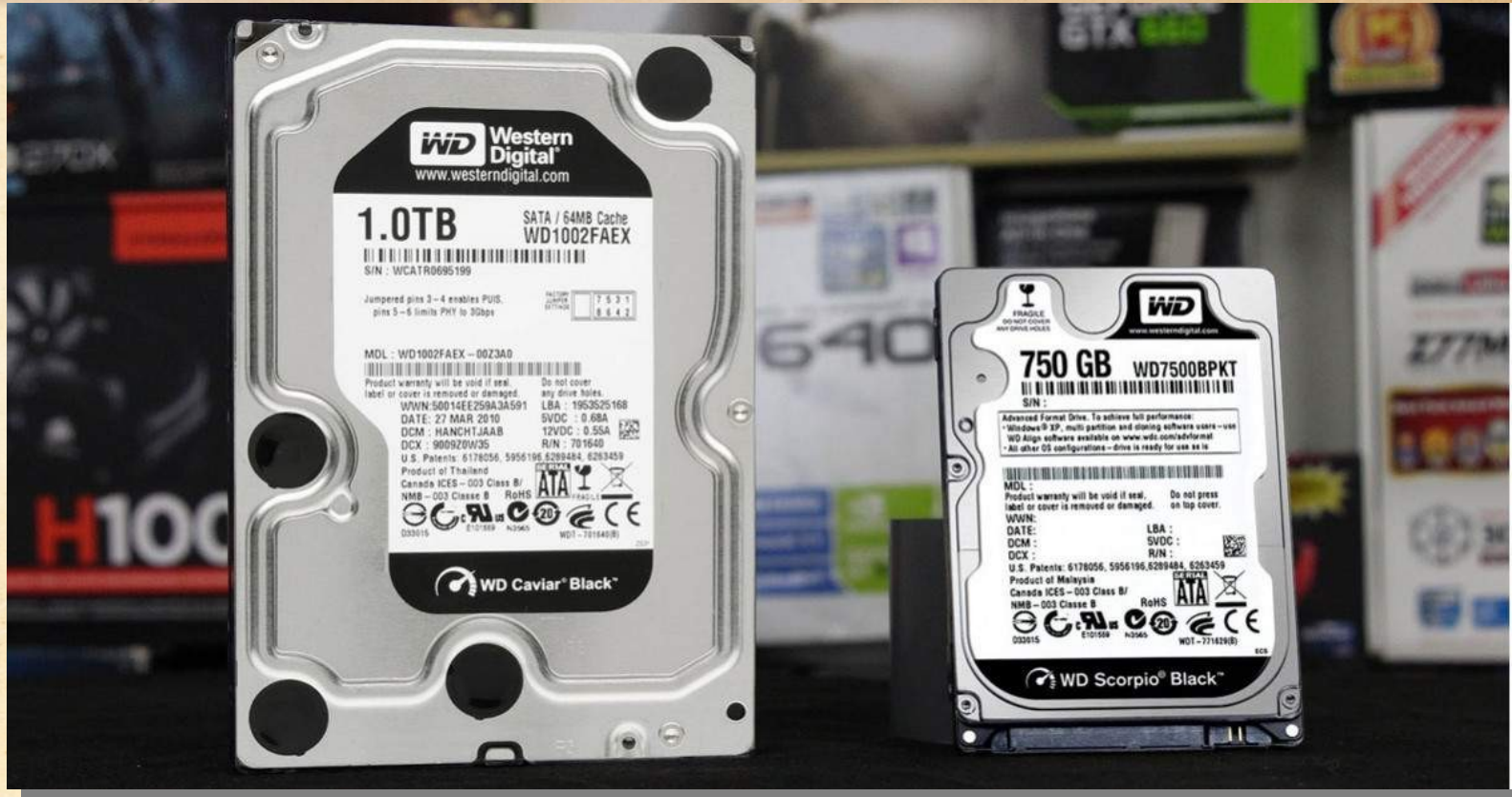
Gambar 6.3 Hard disk internal 3.5 inci dan 2.5 inci
