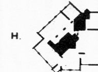
H. Cross Shear Walls & Central Cores
